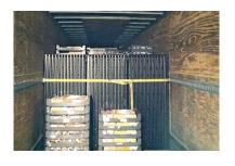
Can be combined with strapping for increased load stability
